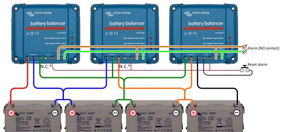
\* Do not connect this terminal. The left reset terminal should only be connected on the battery balancer nearest to system ground.
